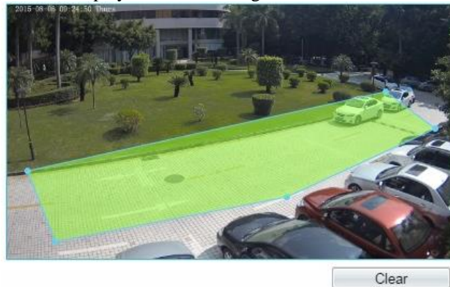
Figure 4-18 Deployment Area Setting Interface
