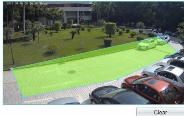
Figure 4-16 Deployment Area Setting Interface
