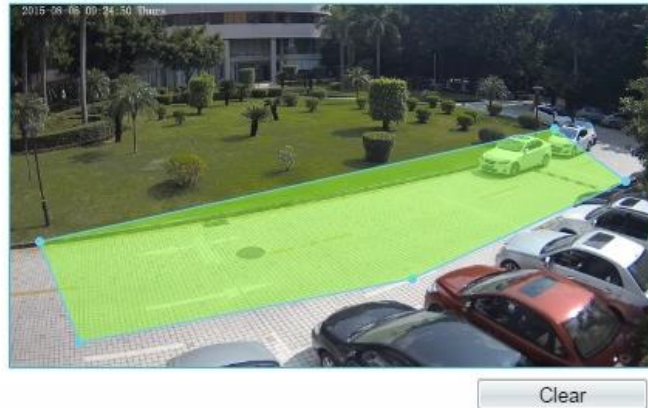
Figure 4-22 Deployment Area Setting Interface
